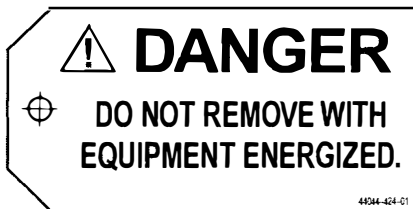
Figure 38: LLI Tag (located on the wiring harness)
